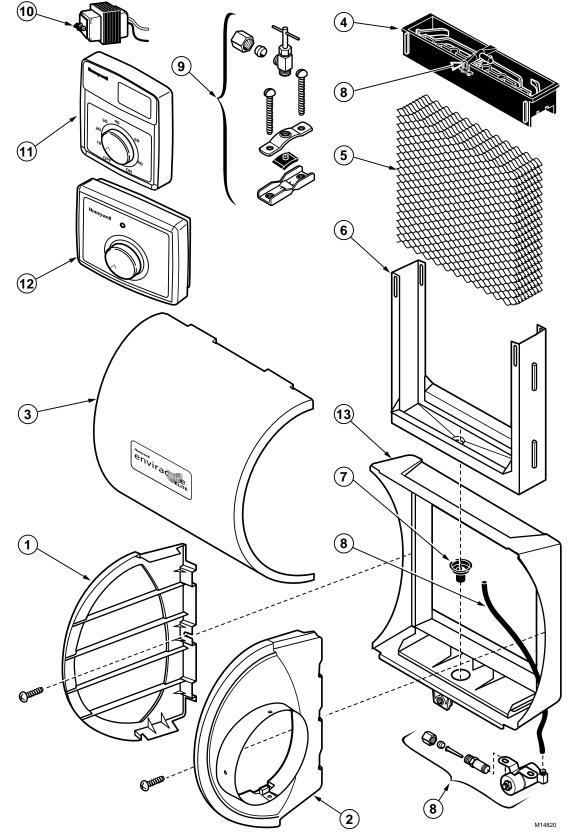
Fig. 6. Exploded view of humidifier parts.
